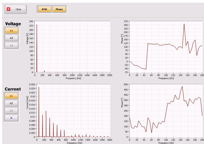
Figure 6. Virtual instrument shows voltage and current spectra for L1 phase
